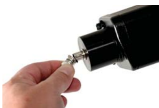
Step 3 - Connect an Ultraprobe to the box
